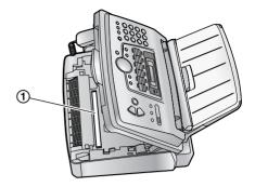
**9** Reinstall the drum and toner unit (①) by holding the tabs.
